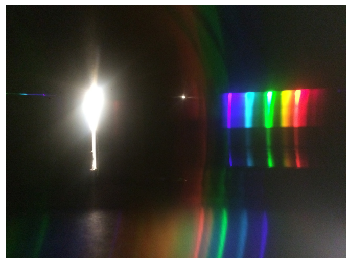
Fluorescent ceiling lamp seen through cookie box spectrometer
