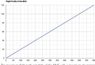
The maximum flight path capability of the MHS, with a maximum downrange distance of 600 meters and a maximum altitude of 120 meters AGL (Graph is NOT drawn to scale). Credit: S.T.E.M. For the Classroom
