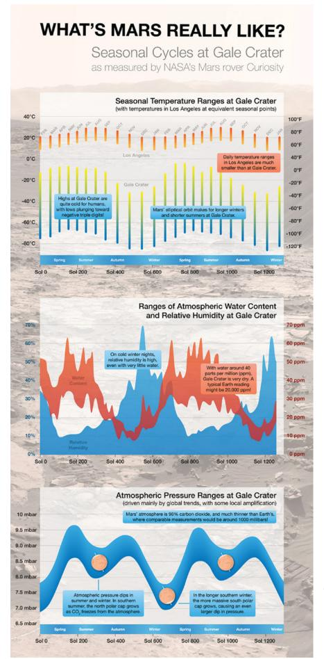
THE WEATHER FROM CURIOSITY: Changing atmospheric conditions as measured by Curiosity since its arrival in Gale Crater. This infographic shows seasonal temperature changes, variations in humidity and atmospheric pressure. A sol is a Martian day, equal to 24 hours 39 minutes 35 seconds. Since a year on Mars is about 687 Earth days, its seasons are correspondingly longer than those on Earth. Credit: NASA/JPL-Caltech
