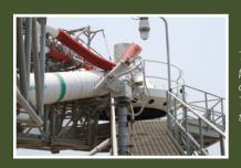
The Beanie Cap served an important purpose – preventing extremely cold oxygen that vented from the External Tank from turning into ice and potentionally damaging the launch vehicle.
