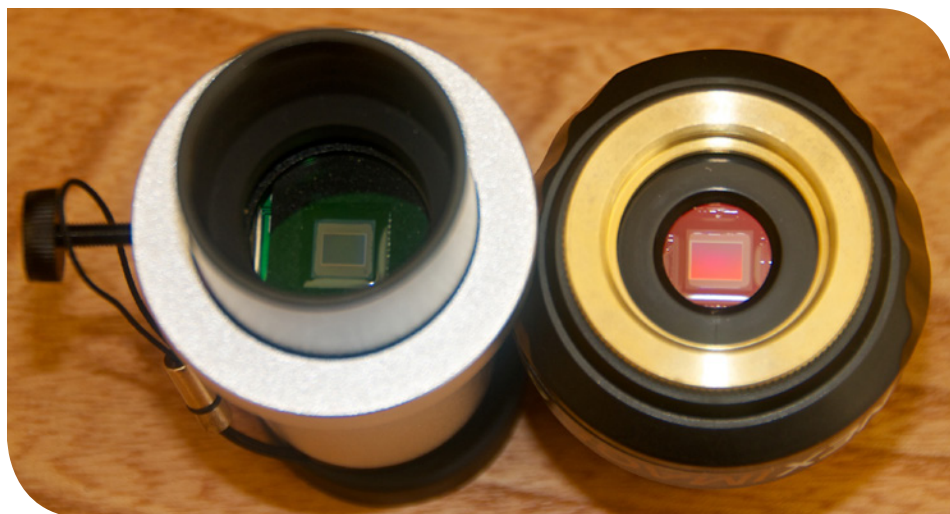
Comparison of the 1.2MP QHY5L-II and 5MP NexImage sensors. Credit: Mike Barrett
