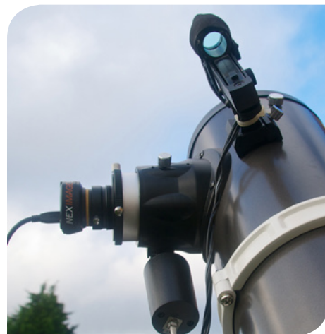
The QHY5L-II guide camera used as a webcam. Credit: Mike Barrett
