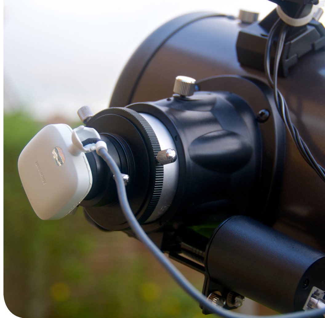
A $10 Xbox webcam can take good images. The most difficult part of the Xbox webcam conversion was opening the casing. Credit Mike Barrett ( www.wired4space.com )
