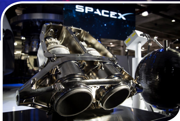
Elon Musk reveals the Dragon V2 (above) that will serve as the first SpaceX spacecraft to be human rated. The capsule will feature eight SuperDraco engines (right) for both launch aborts and for controlled powered landings. Credit: SpaceX
