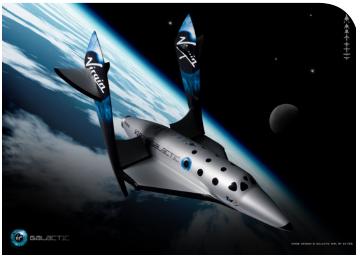
To ensure a safe descent without excessive heating of the spacecraft, SpaceShipTwo's wings will rotate to a 60-degree angle. They will return to horizontal before landing on the Spaceport America runway. Credit: Virgin Galactic
