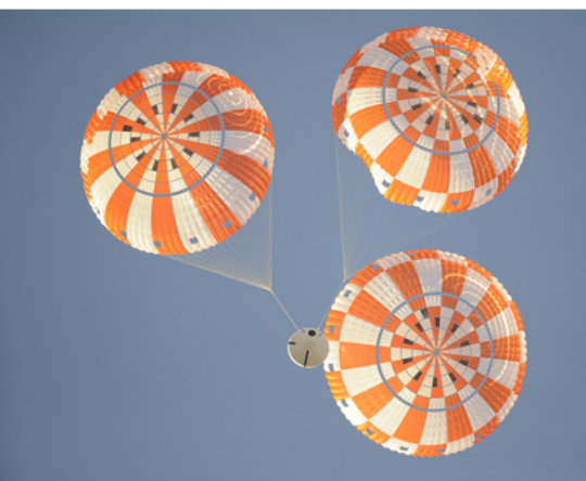
Orion Capsule Parachute Assembly System (above) drop test using the Parachute Test Vehicle (PTV) at the Yuma Army proving grounds in Arizona.
