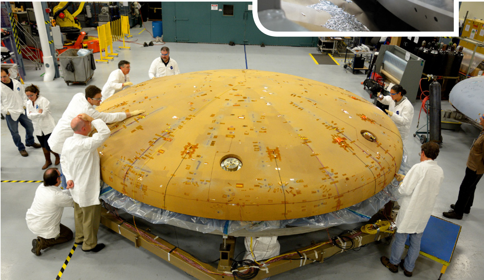
Construction of Orion's heat shield began with Lockheed Martin in Colorado, then was shipped to Boston to have the protective coating applied by Textron Defense Systems.
