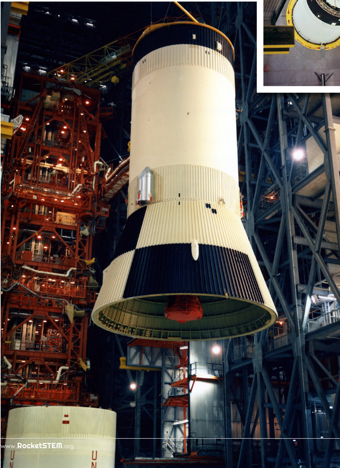
The S-IVB third stage is raised inside the VAB at KSC for mating to the second stage on March 21, 1969.
