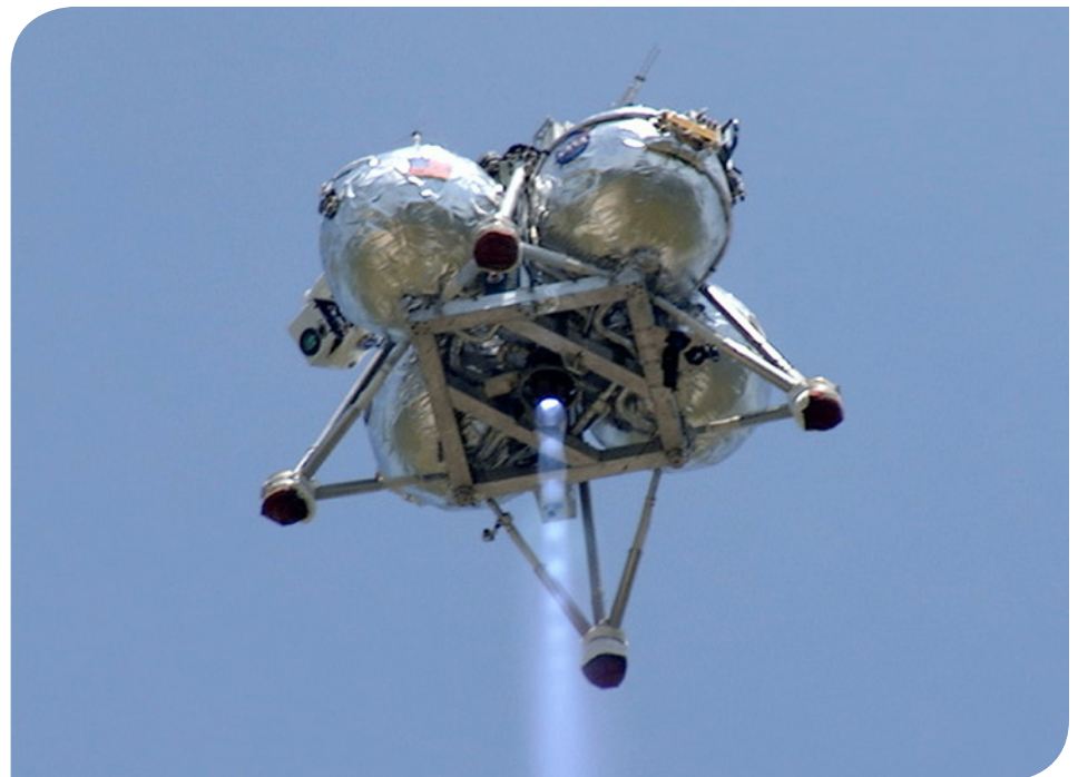
NASA's Project Morpheus prototype lander performs a free-flight test from a launch pad at the north end of the Shuttle Landing Facility at NASA's Kennedy Space Center in Florida.
