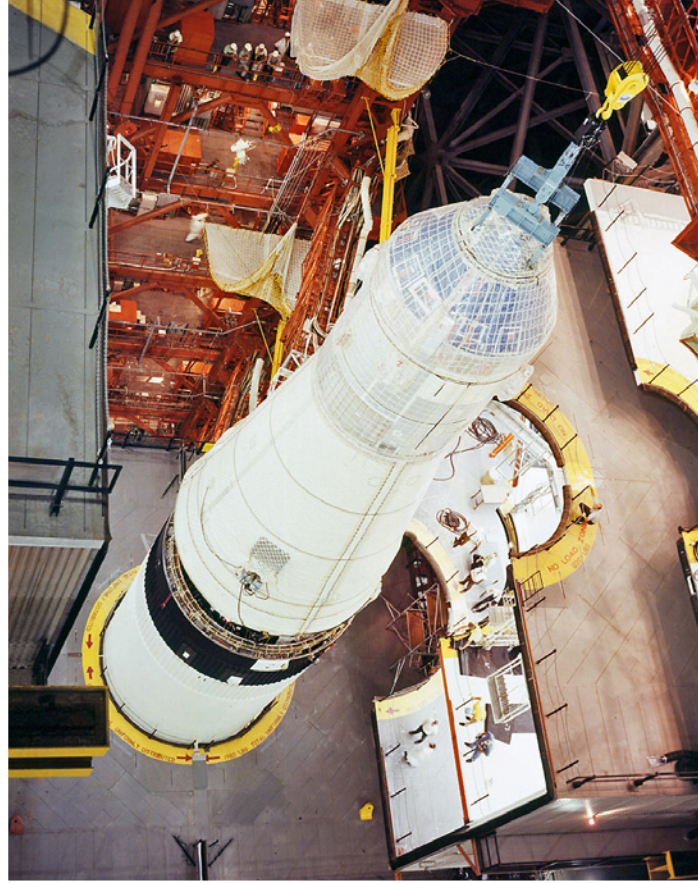
The SLA with the CSM are mated to the Saturn V inside a high bay of the VAB on May 1, 1969.
