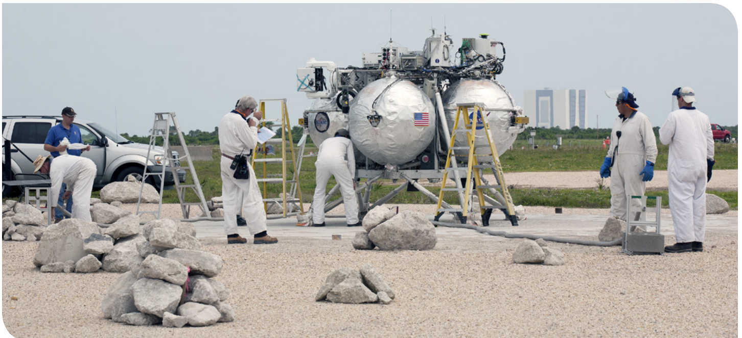
Engineers and technicians check the Project Morpheus prototype lander after it touched down on a dedicated landing pad inside the hazard field at the Shuttle Landing Facility at Kennedy Space Center. Morpheus launched on a free-flight test from a new launch pad at the north end of the facility. Credit: NASA/Kim Shiflett
