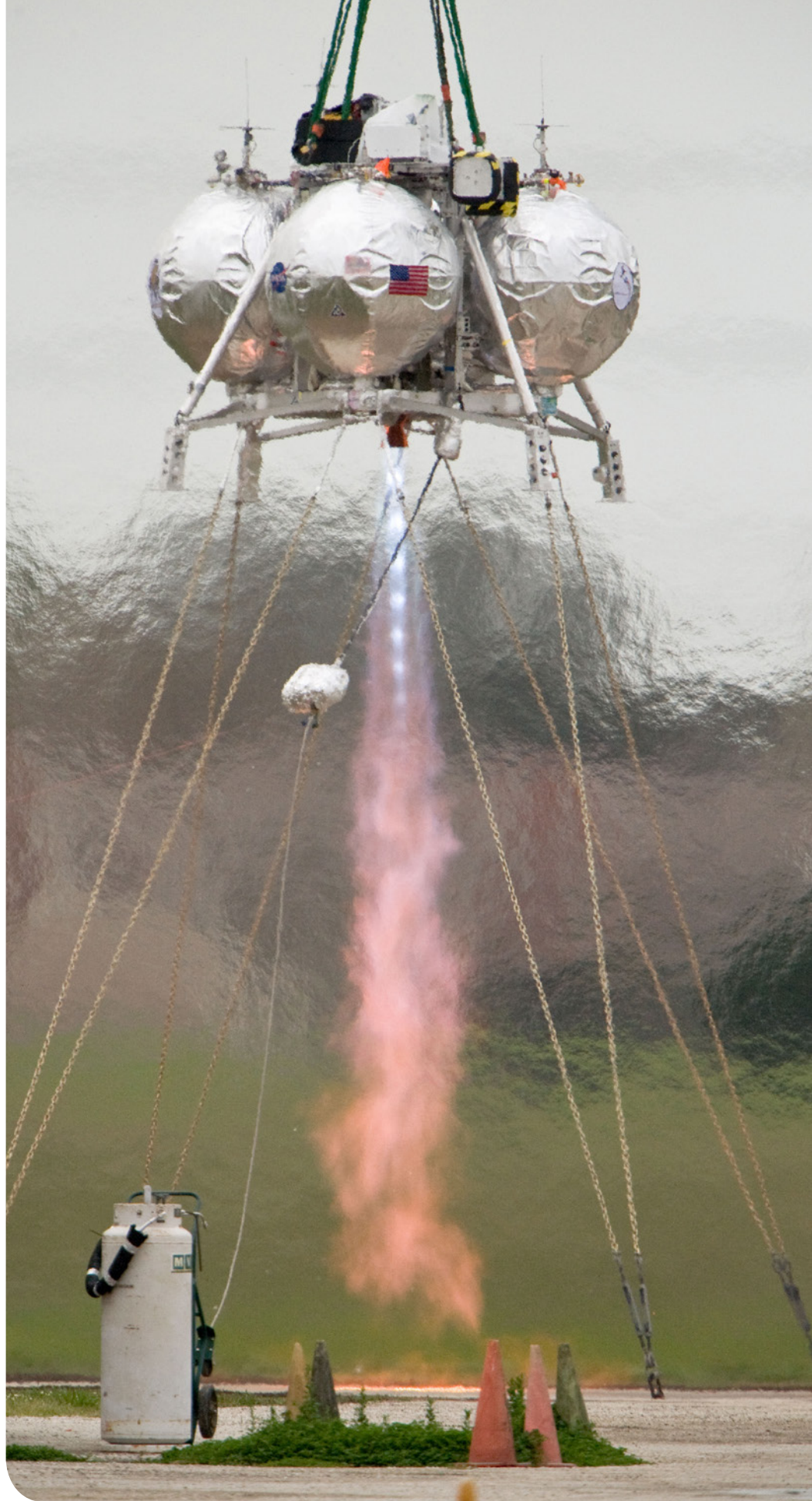
A successful hot fire test of the Morpheus engine in February 2012.
