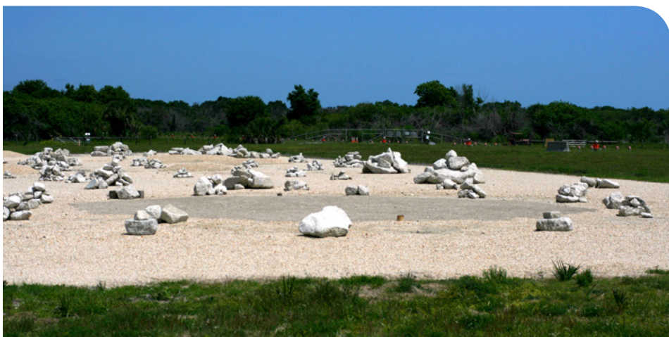
The boulder-strewn hazard avoidance field built to test the Morpheus lander at KSC.
