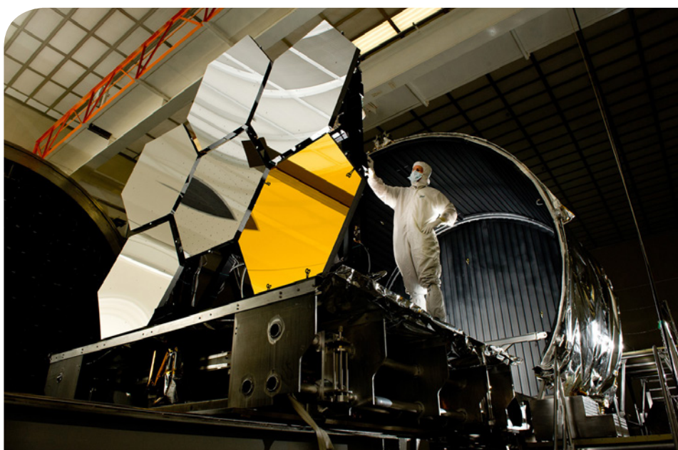
Ball Aerospace lead optical test engineer Dave Chaney inspects six primary mirror segments prior to cryogenic testing. Photo: NASA/MSFC/David Higginbotham
