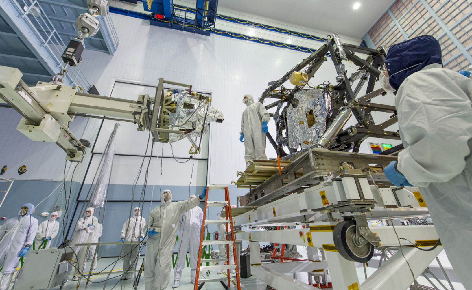
Engineers worked meticulously to implant the James Webb Space Telescope's Mid-Infrared Instrument into the ISIM, or Integrated Science Instrument Module, in the cleanroom at NASA's Goddard Space Flight Center in Greenbelt, Md. Photo: NASA/Chris Gunn
