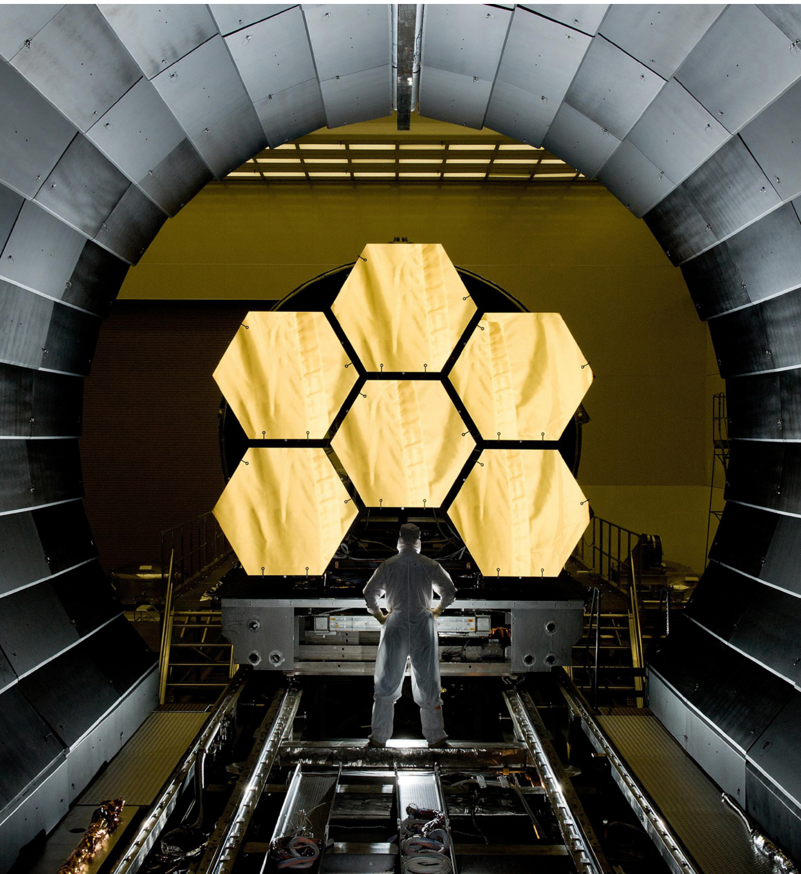
NASA engineer Ernie Wright looks on as the first six flight ready James Webb Space Telescope's primary mirror segments are prepped to begin final cryogenic testing at NASA's Marshall Space Flight Center. This represents the first six of 18 segments that will form the telescope's primary mirror.
