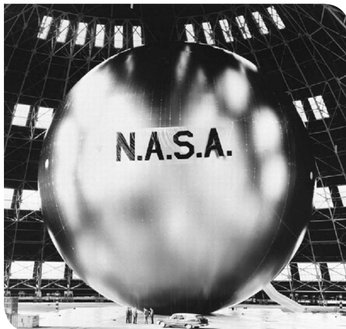
The Echo 2, a rigidized inflatable balloon, was launched into orbit by in 1964. Men and a car are seen at the base of it. Photo: NASA
