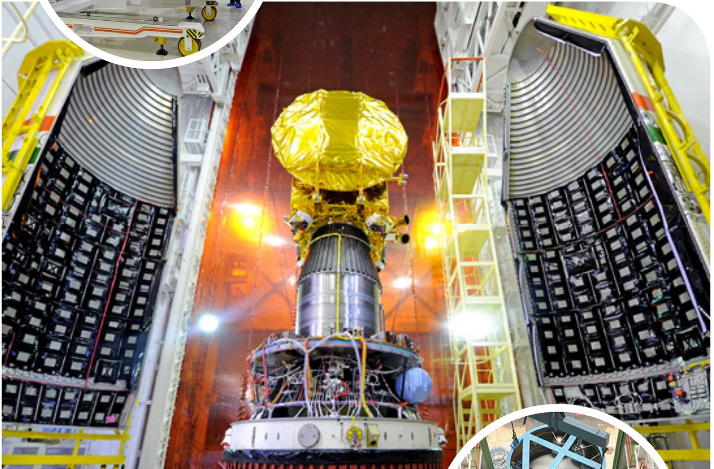
India's Mars Orbiter Mission spacecraft (top) is prepared for a prelaunch test at the Satish Dhawan Space Centre SHAR, Srihairkota in India. The MOM spacecraft (center) is attached to the fourth stage of PSLV-C25 and readied for heat shield closure. The second stage of the PSLV-C25 rocket (bottom) is hoisted into place within the spaceport's Mobile Service Tower.
