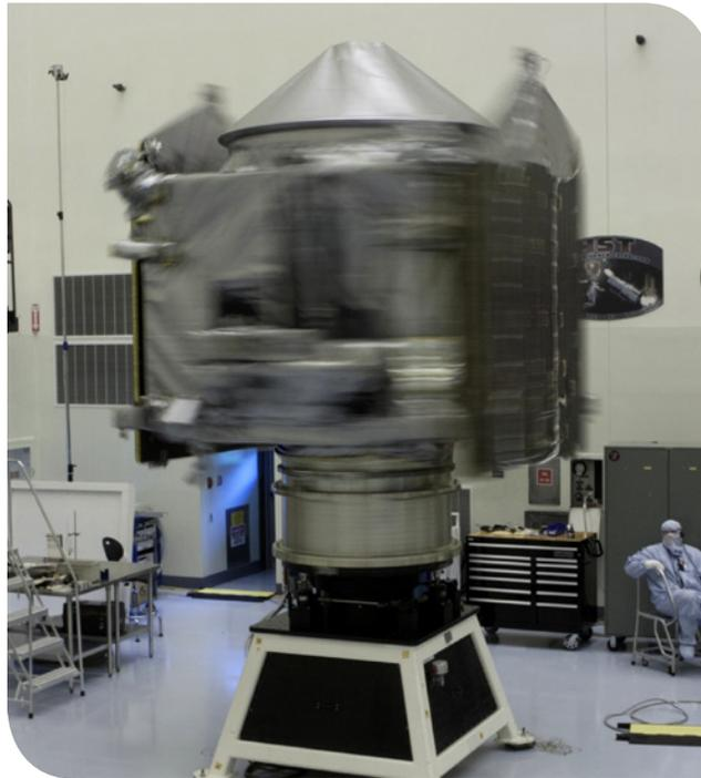
Inside the Payload Hazardous Servicing Facility at Kennedy Space Center in Florida, engineers and technicians perform a spin test of the MAVEN spacecraft. The operation is designed to verify that MAVEN is properly balanced as it spins during the initial mission activities. Photo: NASA/Kim Shiflett
