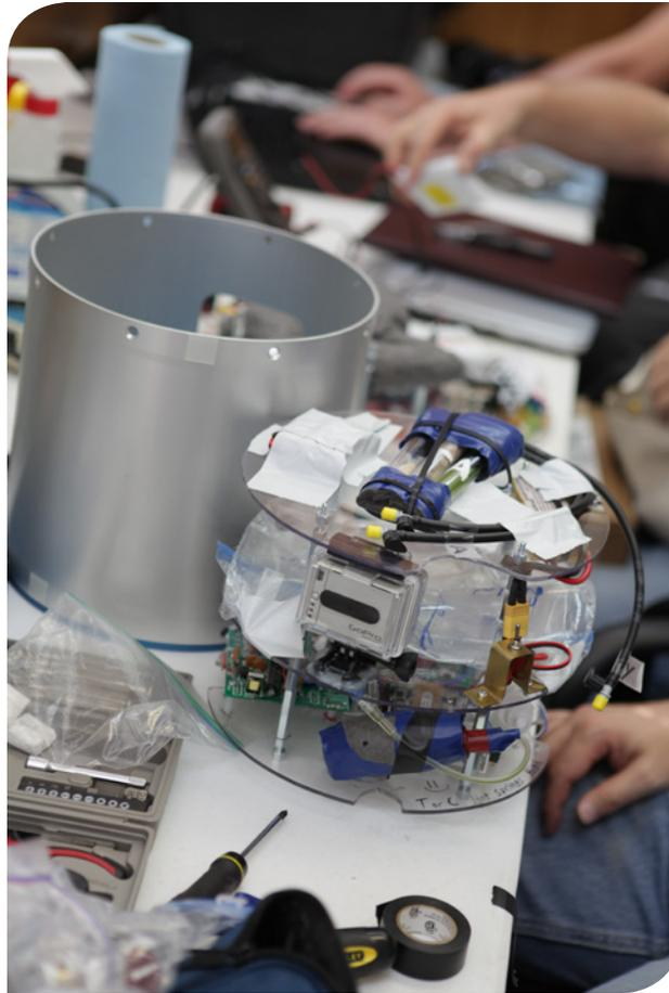
UP Aerospace personnel attached each student team's experiments to Plexiglas shelves that would fit in aluminum payload canisters. Photo: NM Student Launch Program
