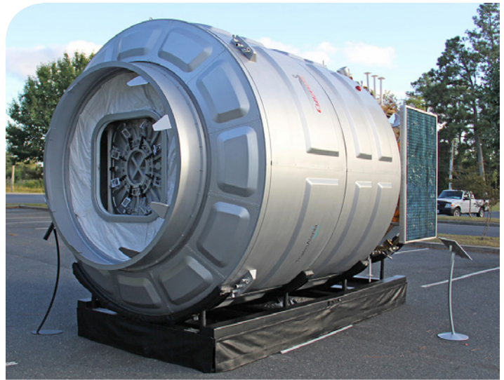
Front view showing docking mechanism and hatch of Cygnus module in this full scale, high fidelity mockup of the Orbital Sciences/Thales Alenia spacecraft gives a feel for it being similar in size to a small room. Image: Ken Kremer
