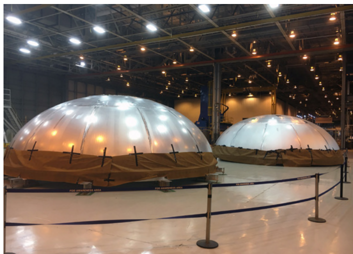
Two fuel tank domes were recently finished for the SLS rocket. One is a qualification article and the other is the actual flight article for the first mission (EM-1) set to launch in 2018. Credit: Chase Clark
