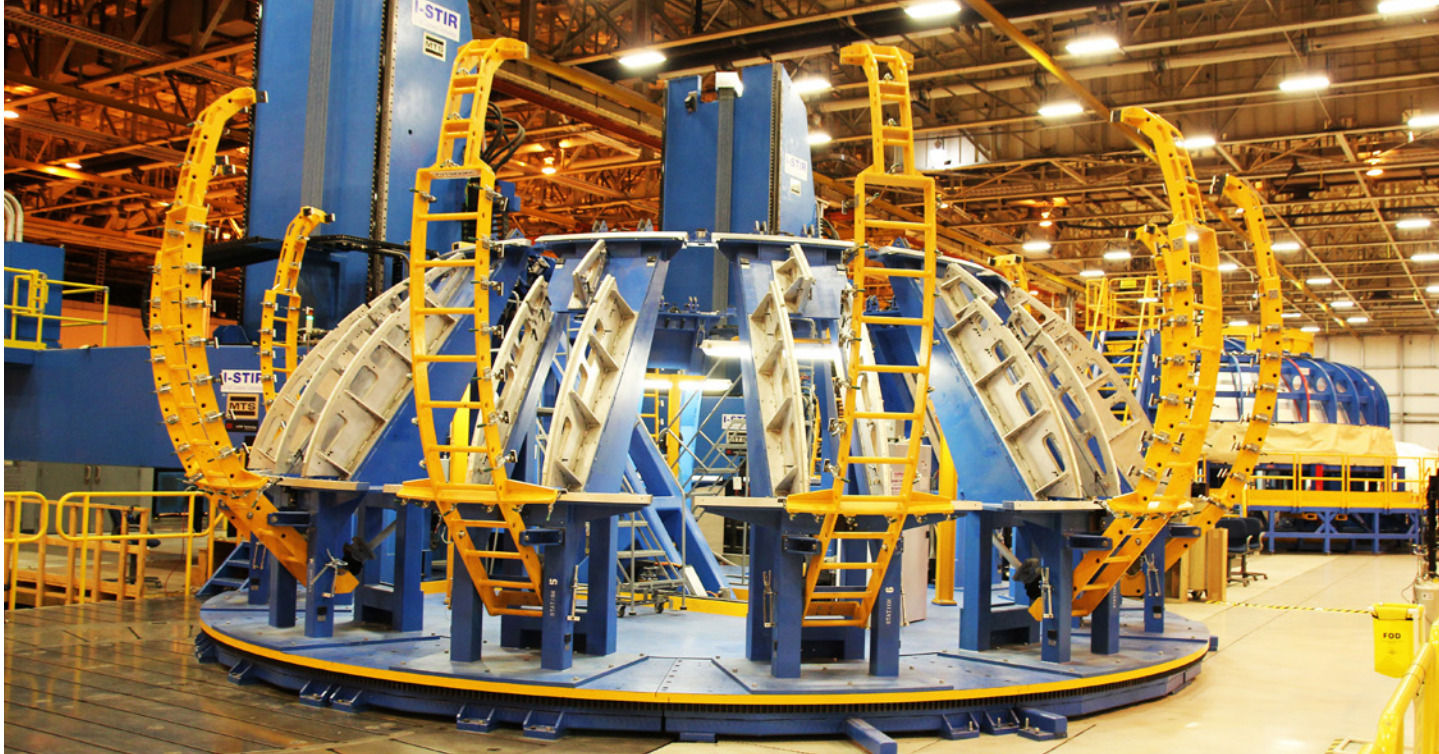
The Gore Weld Tool (foreground) and Circumferential Dome Weld Tool (background) used to fabricate dome segments for the SLS liquid hydrogen and oxygen core stage tanks via vertical friction stir welding operations at NASA's Michoud Assembly Facility in New Orleans. Credit: Ken Kremer
