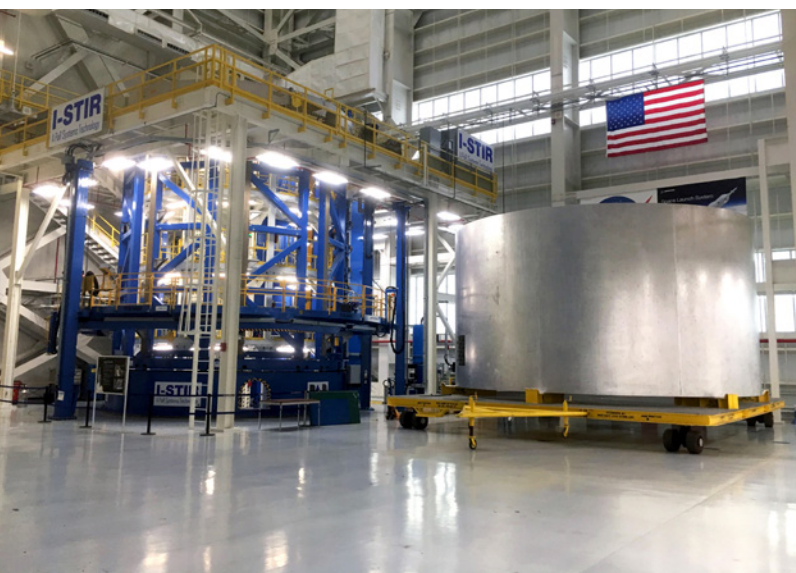
The Vertical Weld Center tool used to fabricate barrel segments for the SLS liquid hydrogen and oxygen core stage tanks via vertical friction stir welding operations at NASA's Michoud Assembly Facility in New Orleans. To the right of the welder is the weld confidence barrel. Credit: Chase Clark
