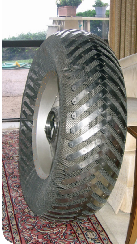
Close-up of the LRV tire exterior, showing the woven piano wire and the titanium treads. A Delco Electronics press photo from the GM Public Relations Department states, "The mesh is steel music wire, 0.033 inches in diameter, crimped at 3/16 inch intervals, cut into 800 32-inch strands, and then woven by hand and shaped to form a tire body. The mesh, containing some 64,000 intersections of wire, is mounted to a spun aluminum disc. The herring-bone tread strips are made of titanium for abrasion resistance. Inside the tire, titanium bumper rings limit deflection of the mesh as the wheel bumps on the lunar terrain." Credit: David Clow
