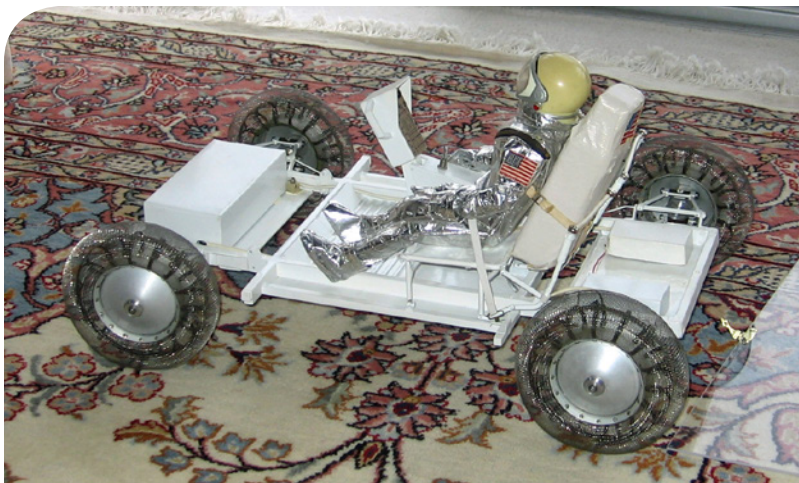
Ferenc Pavlics' original 1/6 scale Lunar Roving Vehicle model, which he drove across the floor of Dr. Wernher von Braun's Huntsville office. The model LRV is folded (right photo) to demonstrate how the full-size Rover could fit into the available space in the Lunar Module descent stage. Credit: David Clow
