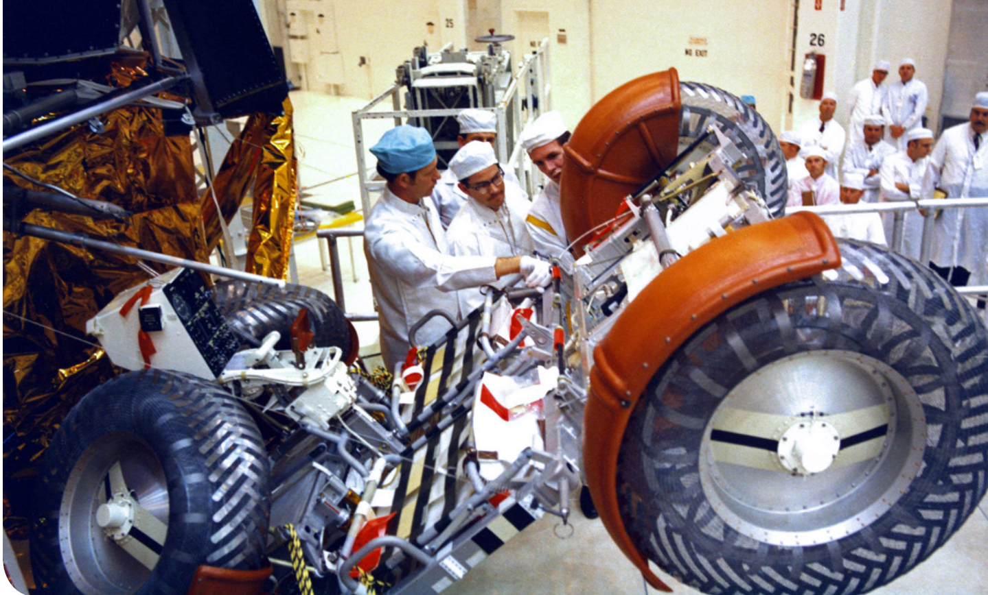
Lunar Rover No. 1, is stowed inside the Apollo 15 Lunar Module at the Manned Spacecraft Operations Building at Kennedy Space Center, Florida. When completely stowed, all four wheels of the LRV are folded against the chassis. Credit: NASA via Retro Space Images
